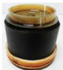
Blocked Hi Lux Fuel Filter.
